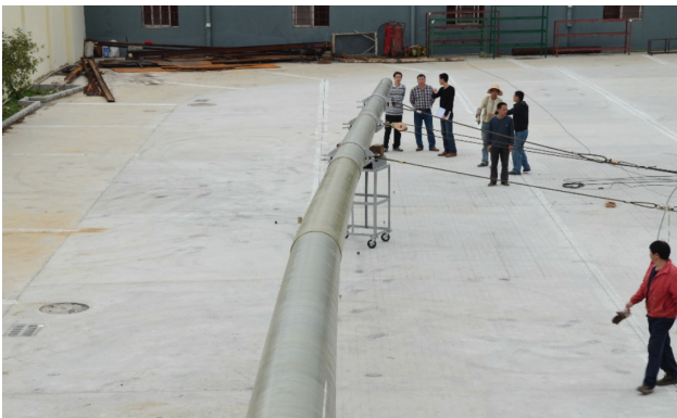
Extreme bending test for utility pole made with BASF's polyurethane product
